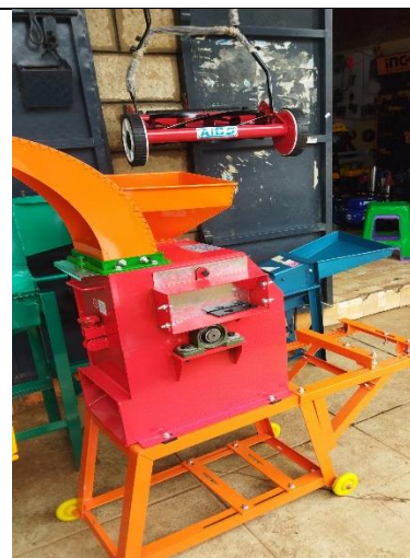
Figure 14: Two in one chaff cutter for dry and wet matter seen at Farady Machinery, Meru
