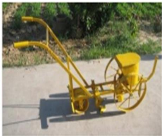
Figure 7: Metallic manual hand-driven seed planter
