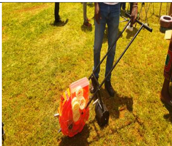
Figure 9: Manual hand-driven seed planter fabricated by FineTouch Africa (@ Ksh. 17,000)
