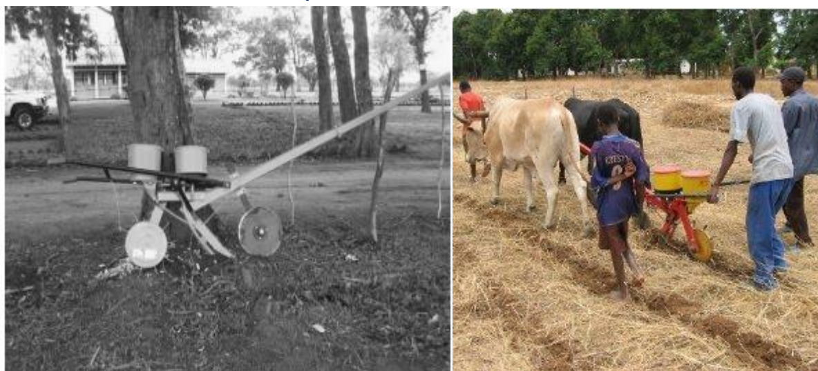
Figure 6: Animal traction direct planter cutting through mulch
