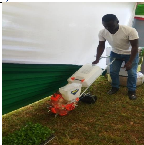
Figure 10: Manual hand-driven seed planter with fertilizer compartment fabricated by FineTouch Africa (@ Ksh. 24,000)
