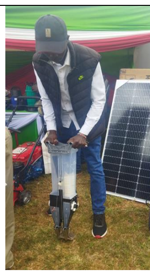
Figure 4: Jab Planter with seed and fertilizer compartment fabricated by Fine Touch Africa (@Ksh. 9,000)
